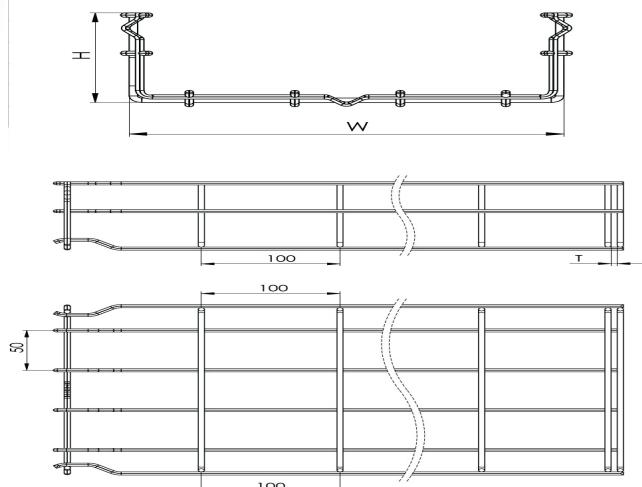
**Wire Mesh Cable Tray (Fast Connect Type) W550mm H100mm T5mm L:3000 SS304****DIMENSIONS**
