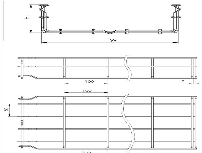
**Wire Mesh Cable Tray (Fast Connect Type) W550mm H35mm T5mm L:3000 EG****DIMENSIONS**
