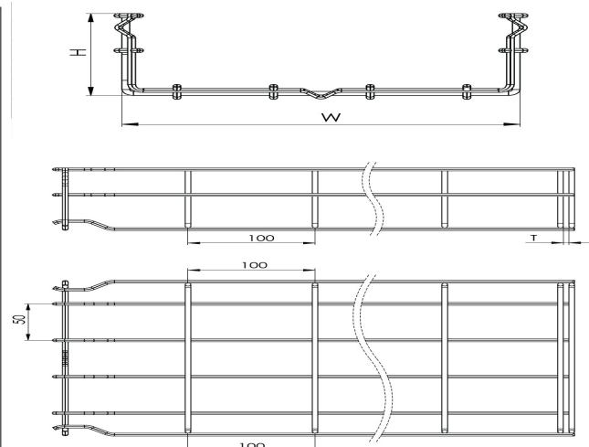
**Wire Mesh Cable Tray (Fast Connect Type) W550mm H35mm T5mm L:3000 HDG****DIMENSIONS**
