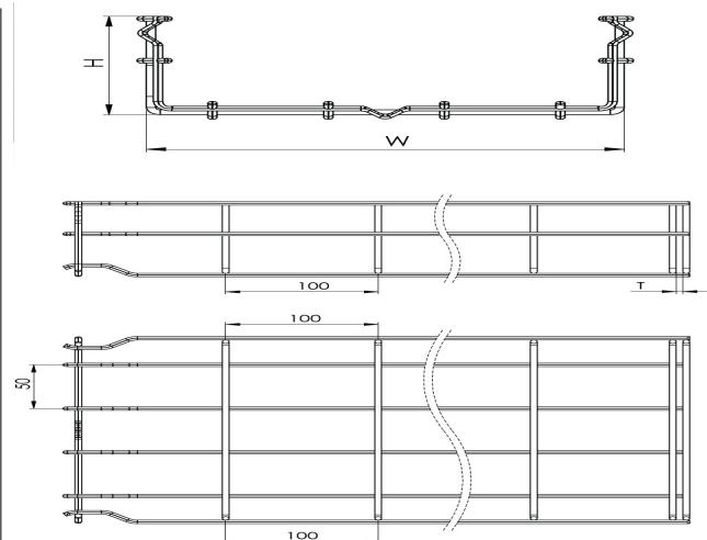
**Wire Mesh Cable Tray (Fast Connect Type) W550mm H35mm T5mm L:3000 SS304****DIMENSIONS**
