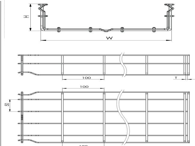
**Wire Mesh Cable Tray (Fast Connect Type) W600mm H100mm T4mm L:3000 EG****DIMENSIONS**
