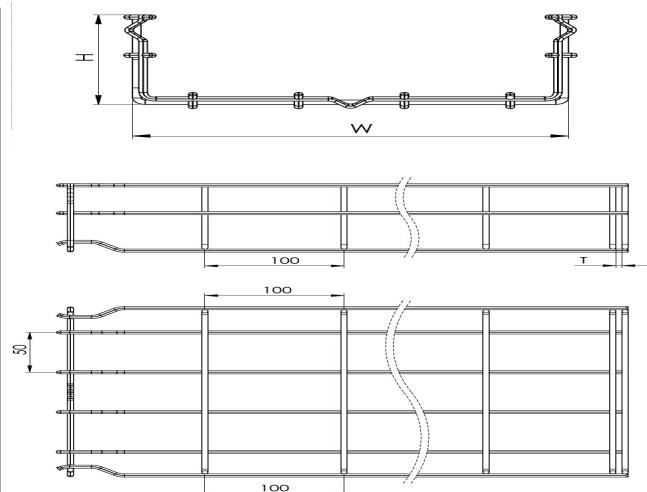
**Wire Mesh Cable Tray (Fast Connect Type) W600mm H35mm T5mm L:3000 SS304****DIMENSIONS**
