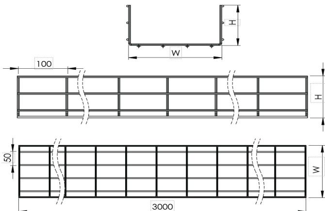
**Wire Mesh Cable Tray (Standard Type) W200mm H100mm T5mm L:3000 SS304****DIMENSIONS**
