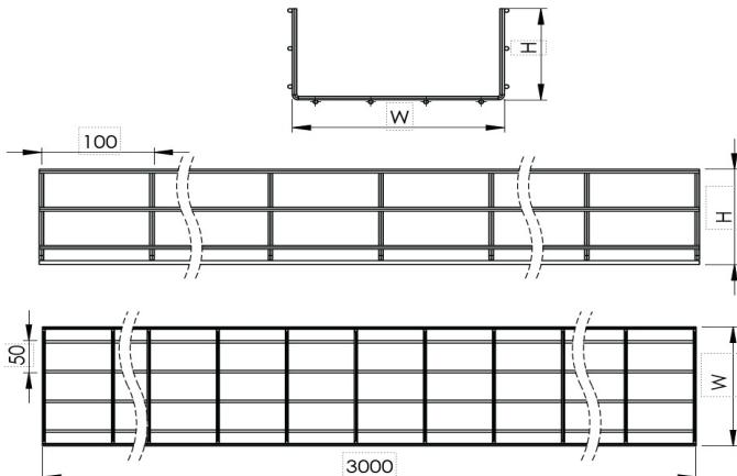
**Wire Mesh Cable Tray (Standard Type) W200mm H35mm T4mm L:3000 EG****DIMENSIONS**
