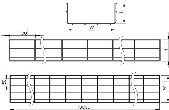
**Wire Mesh Cable Tray (Standard Type) W300mm H35mm T4mm L:3000 EG****DIMENSIONS**
