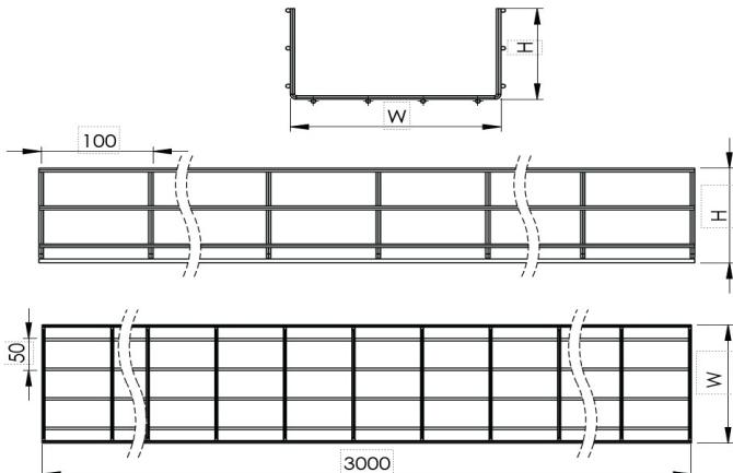
**Wire Mesh Cable Tray (Standard Type) W50mm H60mm T4mm L:3000 SS304****DIMENSIONS**
